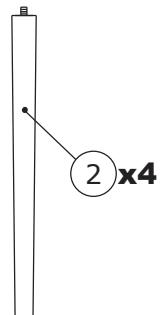
$\varnothing 32 - \varnothing 24 \times 400$  mm
